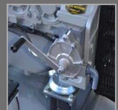
Oil change pump it facilitates oil change
