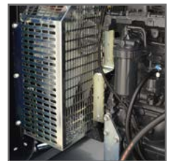
Rotating part guards to prevent injuries to the user
